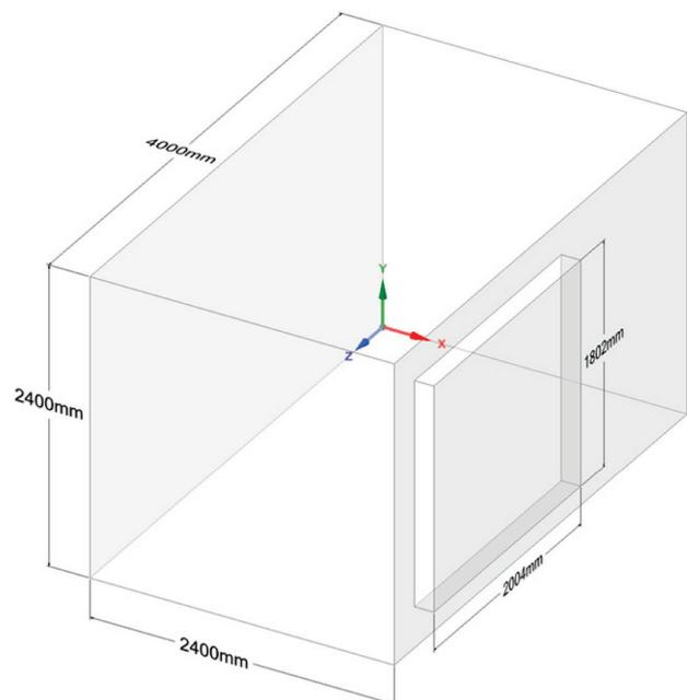
Figure 10: Dimensions of cold room
