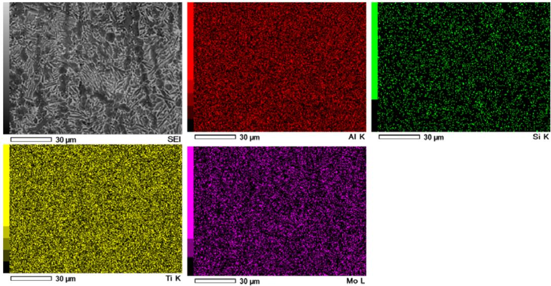
Figure 3: SEM/EDS Phase Mapping of Sample 2 As-Built
