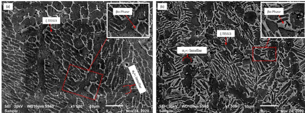
**Figure 1:** SEM image of Non Heat Treated (a) Sample 1 As-Built and (b) Sample 2 As-Built
