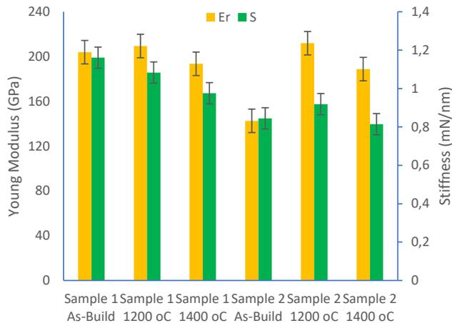
**Figure 6:** Showing the Young Modulus and the Stiffness of both the Samples 1 and Sample 2 As-Built and Heat Treated at 1200 °C and 1400 °C
