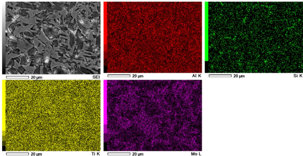
Figure 4: SEM/EDS Phase Mapping of Sample 2 1400 °C
