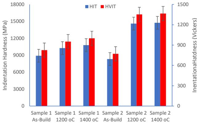
**Figure 5:** Showing the Indentation Hardness in MPa and Vickers Indentation Hardness of both Samples 1 and Sample 2 As-Built and Heat Treated at 1200 °C and 1400 °C
