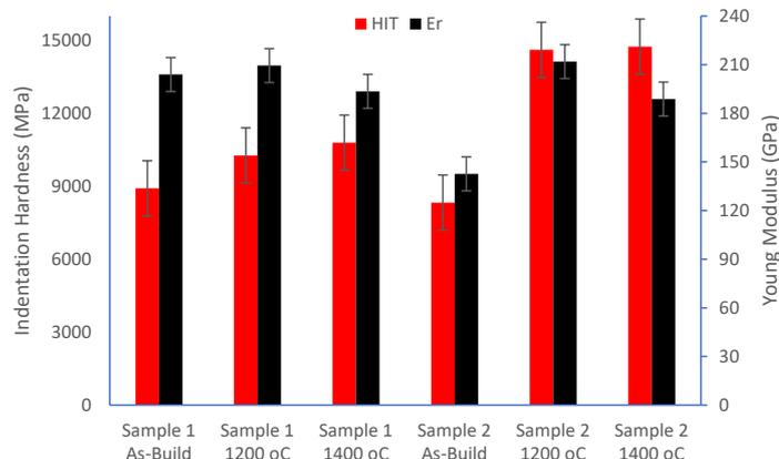
**Figure 7:** Indentation hardness and Young's Modulus of both the Samples 1 and Sample 2 as-built and Heat Treated at 1200 °C and 1400 °C
