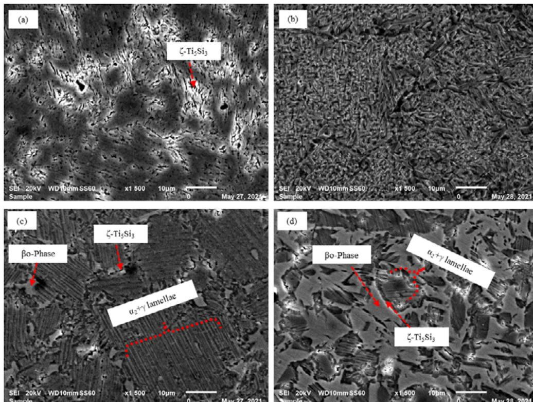
**Figure 2:** SEM image of Heat Treated (a) Sample 1 1200 °C, (b) Sample 2 1200 °C, (c) Sample 1 1400 °C, and (d) Sample 2 1400 °C
