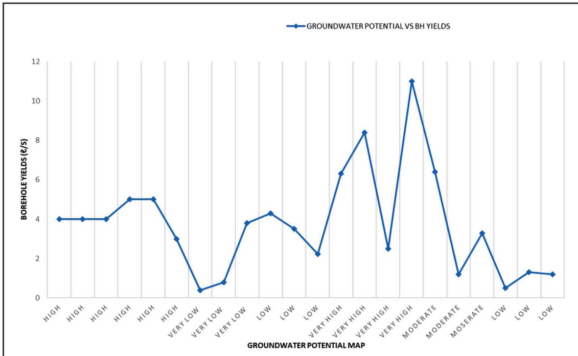
Figure 10: Correlation between produced map and actual borehole yield tests
