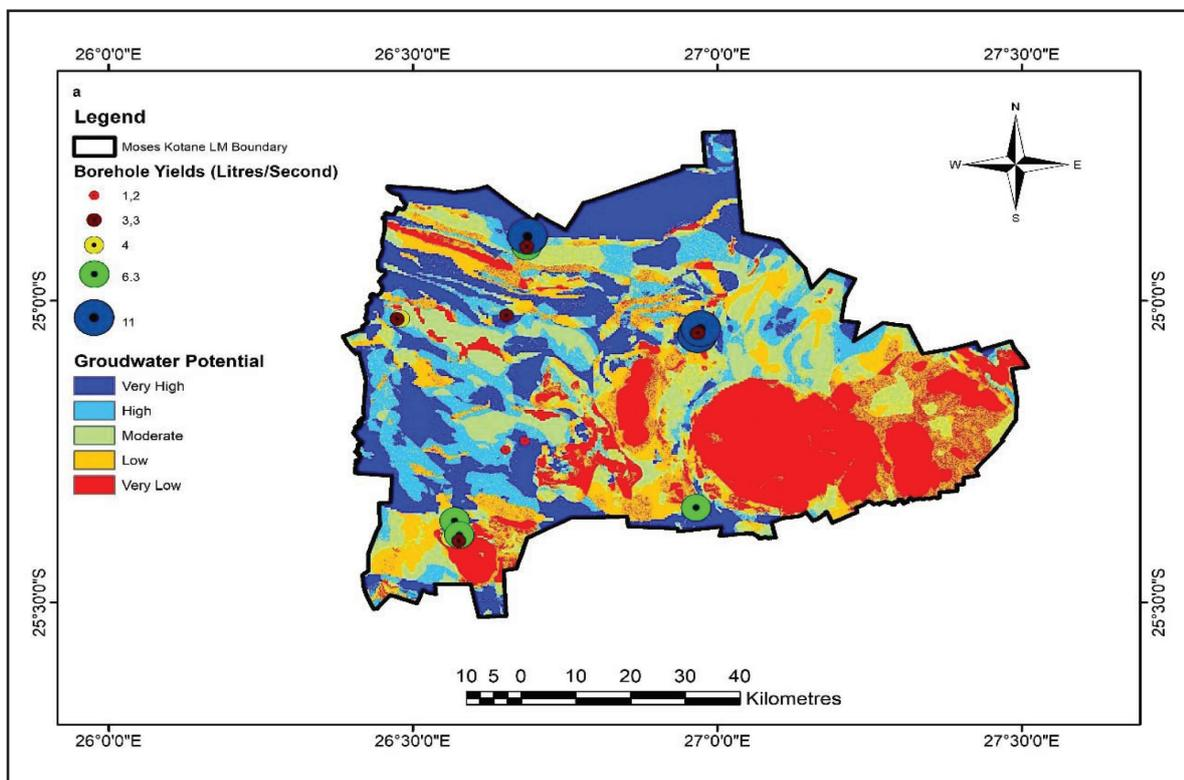
Figure 9: Produced map showing potential zones and actual borehole locations
