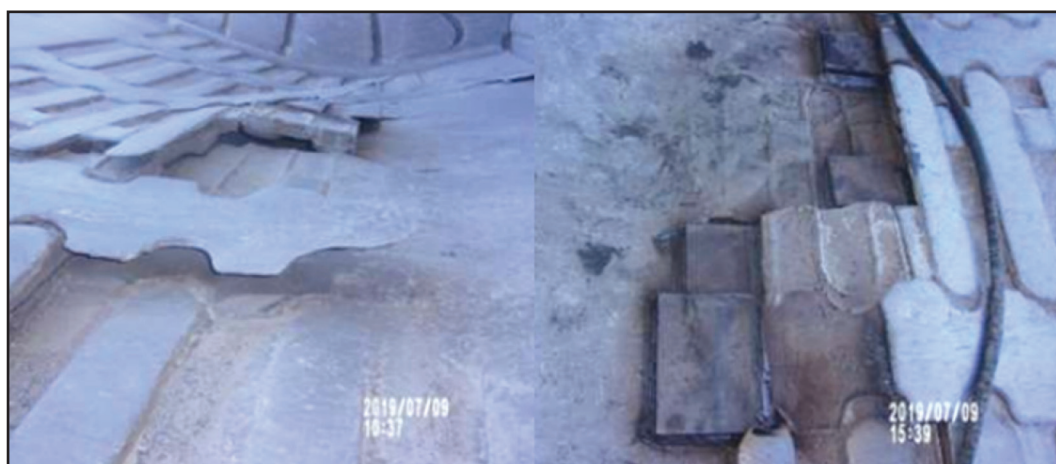
FIGURE 6: Standard wear package damage (LHS), repair (RHS) (JCB-Gearvest (Pty) Ltd, 2019)
