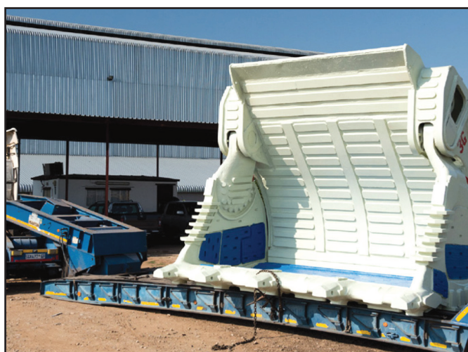
FIGURE 5: RH340 face shovel CCO liner plate repair completed (JCB-Gearvest (Pty) Ltd, 2020)
