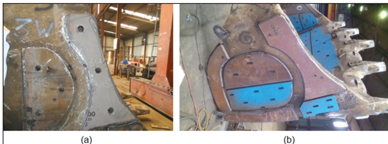
FIGURE 4: Fitment of wear packages (a) AR-plates wear package (b) CCO wear package (JCB-Gearvest (Pty) Ltd, 2018)
