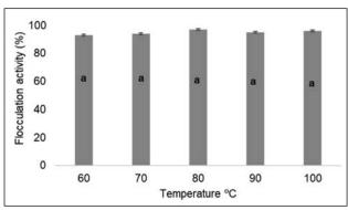
**FIGURE 3:** Effect of heat on flocculation activity of ENMs. Percentage flocculating activities with letter (a) are not significantly (p < 0.05) different.
