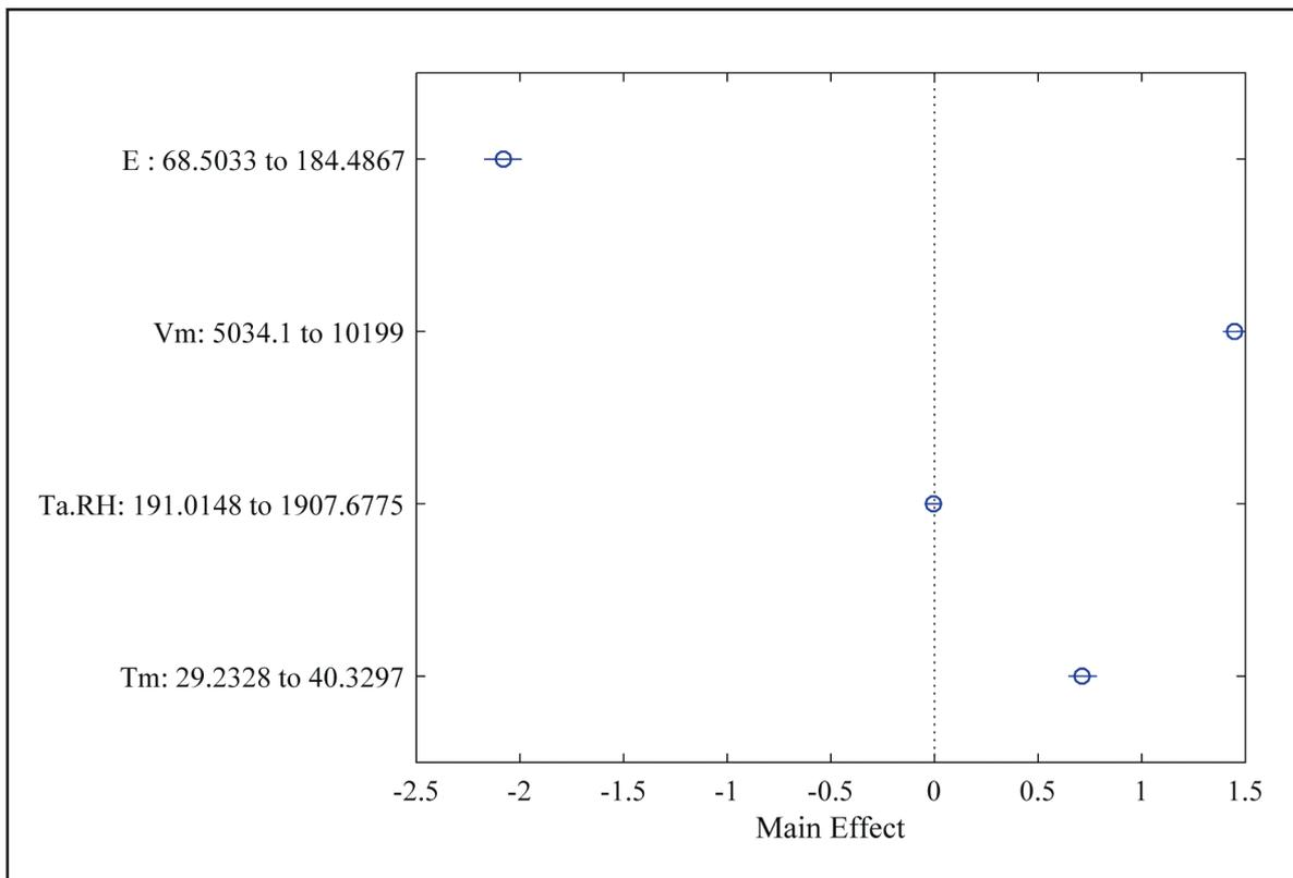
FIGURE 5: Effects of each predictor to the COP of the on-farm DXBMC
