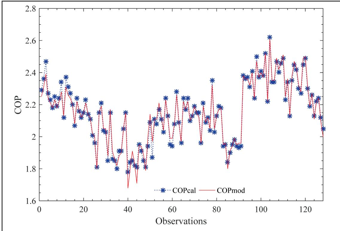
FIGURE 3: Calculated COP and modelled COP for an on-farm DXBMC
